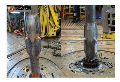
All runs exhibited steady torque responses and trivial levels of vibration. There was also no increase or change in torque signatures when the stabilizers passed through change in formation with different densities. In addition, there was no wear noticed on the RSS, M/LWD or the stabilizer after POOH and all were deemed fit to re-use including the bits.
