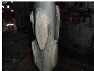
Previously used conventional spiral design string stabilizers were replaced by FIXEDBLADE design stabilizers. In addition, the OD and the placement of the stabilizers were optimized for that particular BHA and application.
