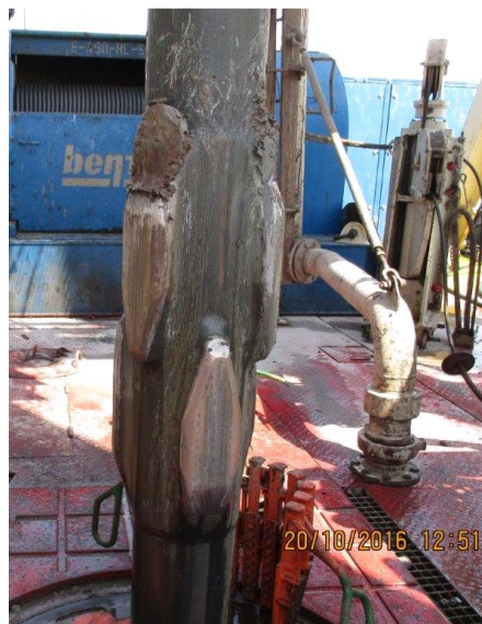
Stabilizers are pulled above the rotary table after drilling 12 ¼" section on the first well
