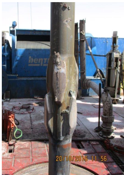
Stabilizers are pulled above the rotary table after drilling 12 ¼" section on the first well
